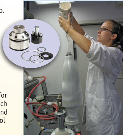
Co-op student Catie Van Fleet begins making a carbon fiber socket using new materials and a tooling and lamination kit she helped develop (see inset).
