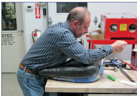
Paul Galloway, director of engineering at PDI, demolds the new lightweight seat for Paralympic rower Oksana Masters – a difficult task because of the seat's shape.
